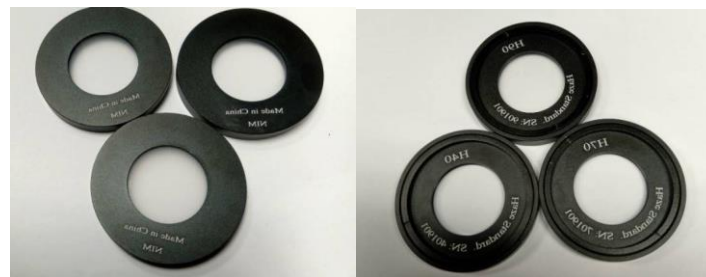
Gambar III.2 Artefak transmittance haze
